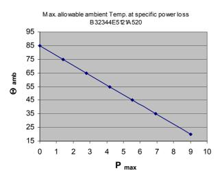
M ax. allo wable ambient Temp. at specific current (rms) B 32344E5121A 520
