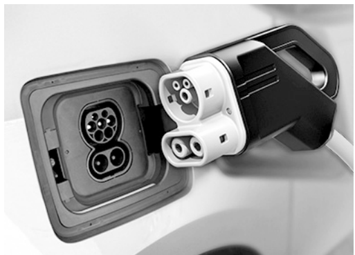
Figure 7 Charging options for electric vehicles and "vehicle connection to a Combo 2 fast charging station"
